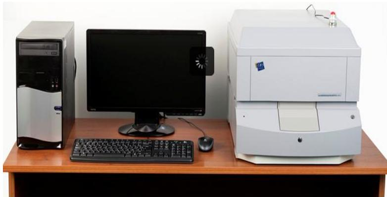
"SPECTROSCAN MAKC-GV" WDXRF spectrometer determines elements from Na (Sodium) to U (Uranium) in solids, liquids or powders, in solutions and thin films, deposits on filters.
